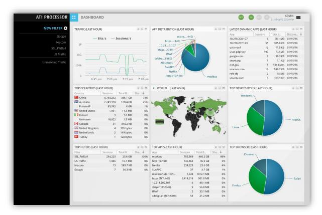
The CloudLens<sup>™</sup> Packet Processing with AppStack Dashboard features easy to use graphical displays and offers an overview of the network traffic map. The administrator can quickly see where the traffic is coming from, what are the most active applications, and countries in a certain period of time. Which operating systems, and devices are active on the network.
