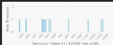
Fig. 4: Humans are usually more random in their key presses than even a sophisticated bot. By examining the velocity and cadence of a human's key presses, Akamai can further determine if a user is a bot.
