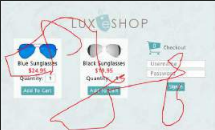
Fig. 3: Sophisticated bots will try to hide by triggering mouse moves. This is designed to emulate a user's interaction. However, after a certain number of moves, a pattern will emerge. Akamai can detect these patterns to identify a bot.
