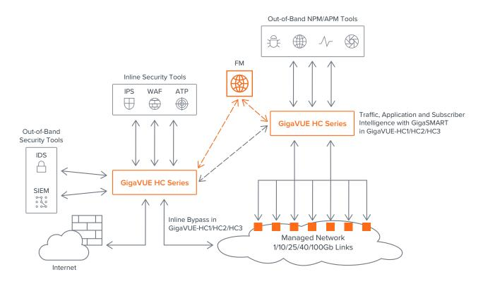
GigaVUE HC Series is used to provide visibility for active and passive security as well as network and application monitoring.
