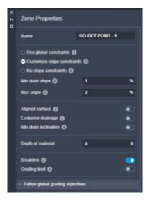
Zone properties identify the parameters in which the Optimizer is allowed to iterate to find a solution.
