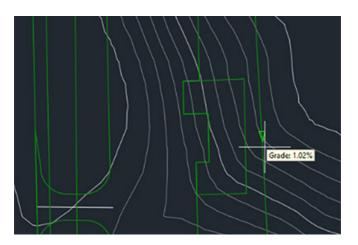
Feature line slopes can be adjusted to create proper drainage.
