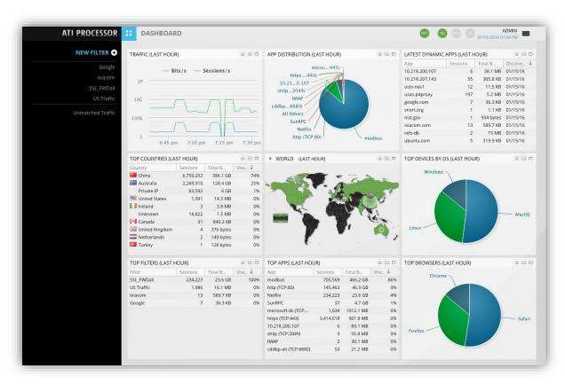
The CloudLens™ Packet Processing with AppStack Dashboard features easy to use graphical displays and offers an overview of the network traffic map. The administrator can quickly see where the traffic is coming from, what are the most active applications, and countries in a certain period of time. Which operating systems, and devices are active on the network.
