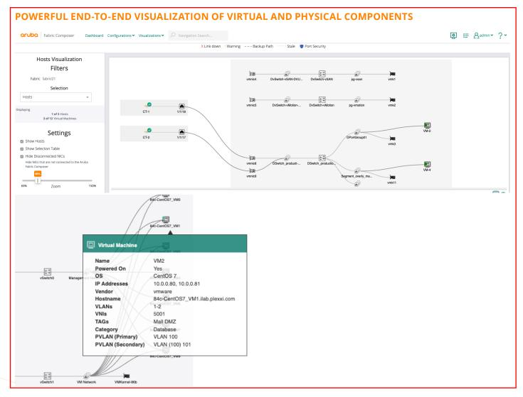
Using the Aruba Fabric Composer Host View, administrators can easily see end-to-end connectivity between Virtual Machines, Port Groups, vSwitches, and Physical NICs to visualize how they are connected to Aruba CX switch ports.
