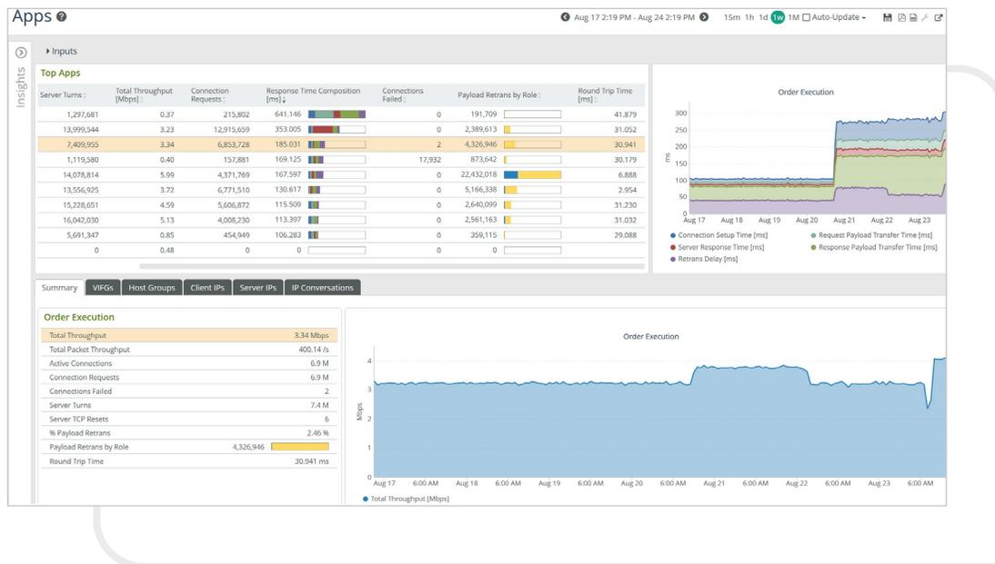
**Figure 2:** AppResponse provides easy-to-use analytics that show all relevant information for troubleshooting. This shows the top applications, the response time composition, and summary info for a given app. Additional drill-down investigations available by clicking on the tabs.
