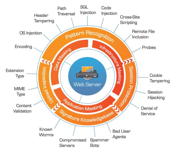
**dotDefender** is a software Web Application Firewall (WAF), boasting enterprise-class security, advanced integration capabilities, easy maintenance and low total cost of ownership (TCO). **dotDefender** is the perfect choice for protecting your website against hackers and complying with PCI DSS regulations.
