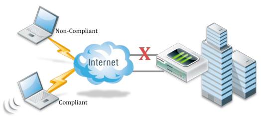
Devices deemed noncompliant by FortiGate device at head-end result in denial of access or warning to the user.
