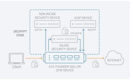
Figure 2: A10 Thunder SSLi or CFW devices can decrypt traffic for a variety of security products, including inline, non-inline (passive/TAP) and ICAP enabled devices.
